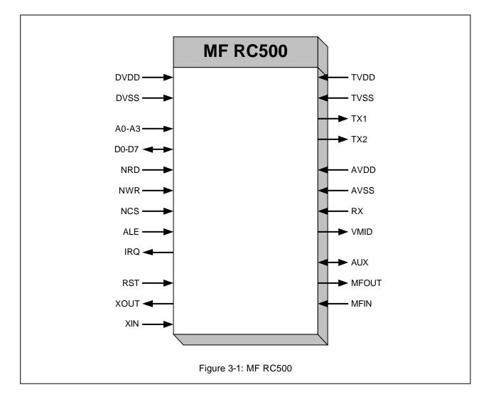
The device operates with 3 individual power supplies for best performance in terms of EMC behaviour and signal de-coupling. This gives outstanding RF performance and also maximum flexibility to adapt to different operating voltages of digital and analog part.
