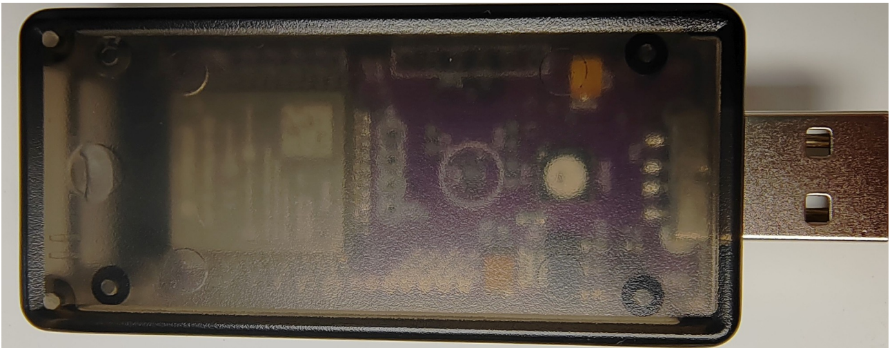
ESP32-DEVKIT12C-RGB mounted in semitransparent USB enclosure
