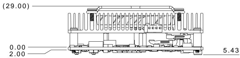
With Heat Spreader and Active Cooling (Part No: COM-TGUC6-HSP01 and COM-FAN02)
