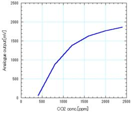
Fig 4. Converting analogue output to CO2 concentration
