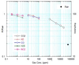
Fig 3. Cross sensitivity (SB-AQ6A)
