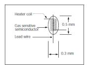
Fig 1. Sensing element
