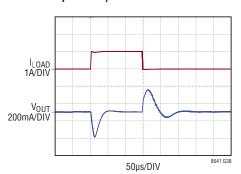
FRONT PAGE APPLICATION 300mA (Burst Mode OPERATION) TO 1.3A TRANSIENT  $12V_{IN}, 5V_{OUT} \\ C_{OUT} = 47 \mu F$
