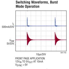
Figure 3. Burst Mode Operation
