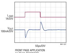
FRONT PAGE APPLICATION 1A TO 2A TRANSIENT  $12V_{IN}$ ,  $5V_{OUT}$   $C_{OUT} = 47\mu F$
