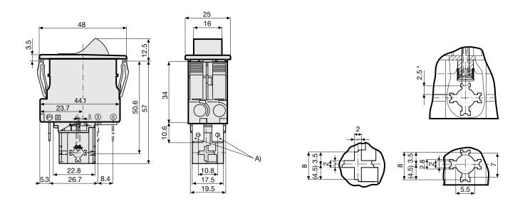
A) Quick connect terminal, IEC 61210, A6.3-0.8 mm
