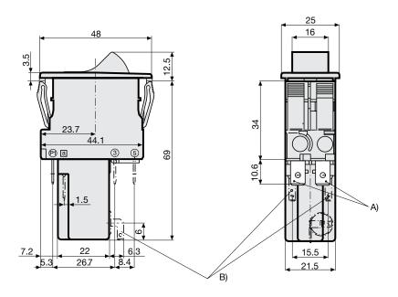
A) Quick connect terminal, IEC 61210, A6.3-0.8 mm B) Quick connect terminal, IEC 61210, A2.8-0.8 mm
