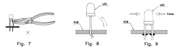
7. No stress shall be applied on the LED during soldering to prevent damage.
