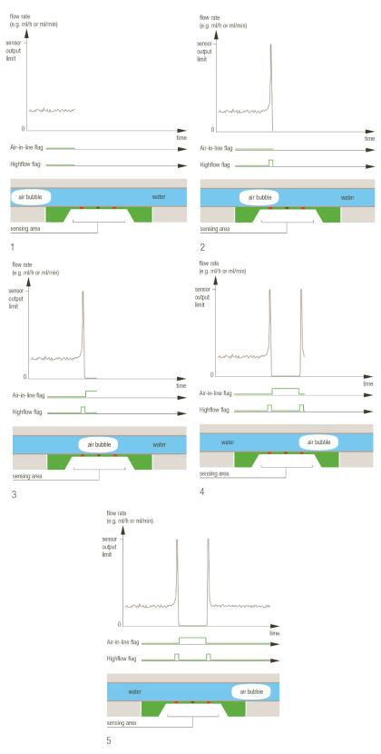
**Figure 3:** Detection of air-in-line events with the SLF3S-4000B. The graphs illustrate the air-in-line and high-flow flags while a bubble is passing though the sensor from left to right.
