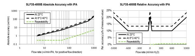
Figure 2: Left: Liquid flow sensor accuracy and repeatability across the flow range of the SLF3S-4000B. Relative error in ±% of measured value for IPA. Right: Liquid flow sensor accuracy and repeatability across the positive flow range of the SLF3S-4000B. Absolute error in ml/min for IPA.
