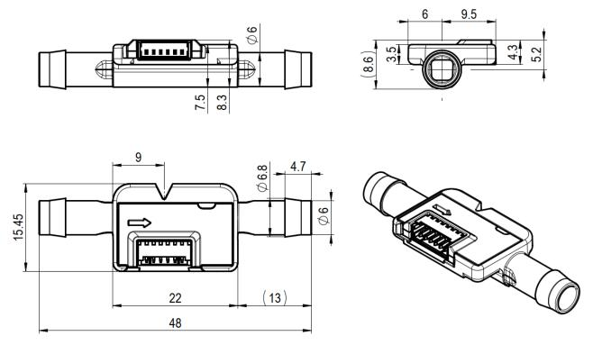
Figure 4: Dimensions of SLF3S-4000B (all dimensions in mm)
