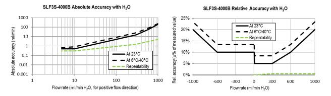
Figure 1: Left: Liquid flow sensor accuracy and repeatability across the flow range of the SLF3S-4000B. Relative error in  $\pm \%$  of measured value for H<sub>2</sub>O. Right: Liquid flow sensor accuracy and repeatability across the positive flow range of the SLF3S-4000B. Absolute error in ml/min for H<sub>2</sub>O.
