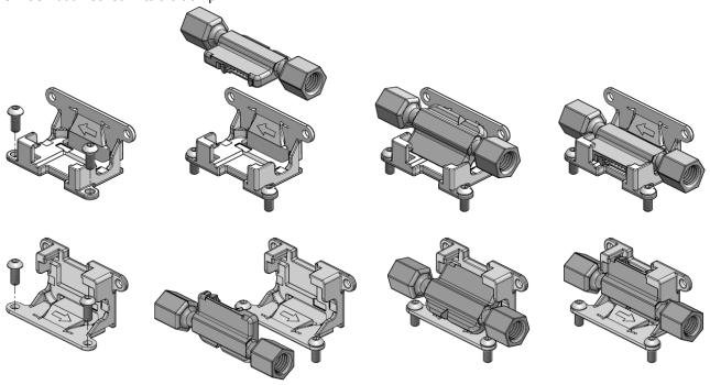
Figure 5: Mounting guidelines for the SLF3S-4000B sensor into the SLF3x mounting clamp
