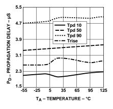
Figure 14. Propagation Delay vs. Temperature.
