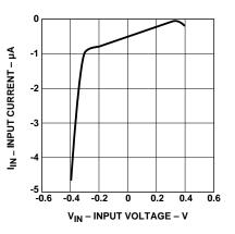
Figure 11. Input Current vs. Input Voltage.
