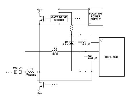
Figure 17. Recommended Supply and Sense Resistor Connections.
