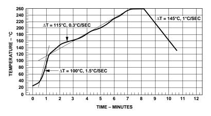
(NOTE: USE OF NON-CHLORINE ACTIVATED FLUXES IS RECOMMENDED.)
