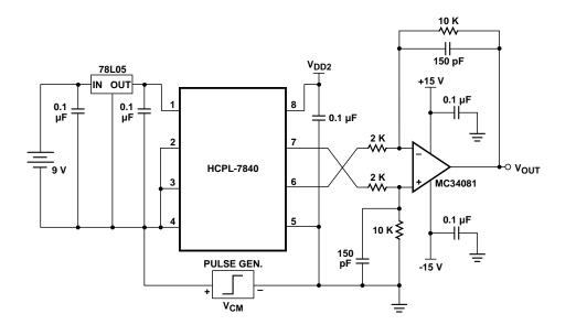
Figure 16. CMTI Test Circuits.
