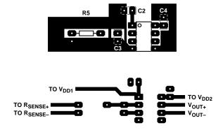
Figure 19. Example Printed Circuit Board Layout.
