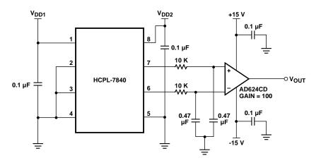
Figure 1. Input Offset Voltage Test Circuit.
