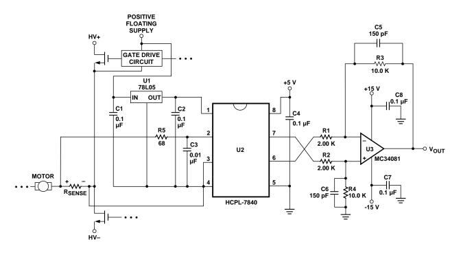
Figure 18: Recommended Application Circuit.
