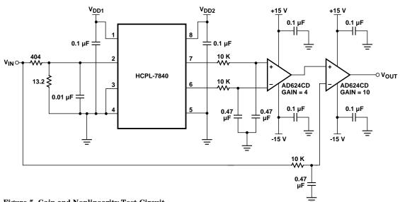
Figure 5. Gain and Nonlinearity Test Circuit.
