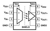
The product can also be used for general analog signal isolation applications requiring high accuracy, stability, and linearity under similarly severe noise conditions. For general applications, we recommend the HCPL-7840 (gain tolerance of  $\pm$  5%). The HCPL-7840 utilizes sigma delta ( $\Sigma$ - $\Delta$ ) analog-to-digital converter technology, chopper stabilized amplifiers, and a fully differential circuit topology fabricated using
