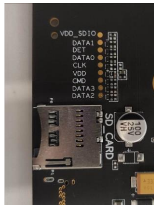
Figure 23: Pin Assignment of SD Card Connector J1401
