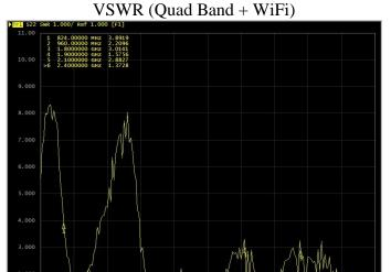
Tested with 15cm cable length - RG174 with SMA male
