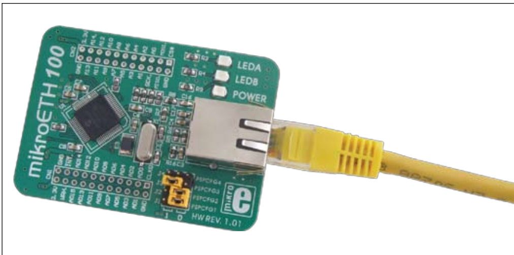
Figure 4: mikroETH 100 connected to the Ethernet cable
