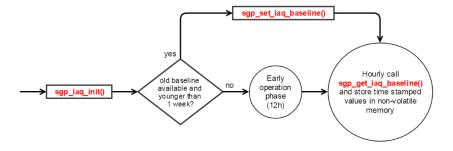
Call  $sgp\_iaq\_init()$  to reset all SGP baselines. The initialization takes up to around 15 seconds, during which  $sgp\_iaq\_measure()$  output will not change.
