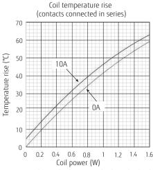
Note: When each contact is used independently, above graph shall be read; same voltage is applied on 2 coils, coil power is sum of 2 coils, applied current 10A is 10A apply on each contact set.
