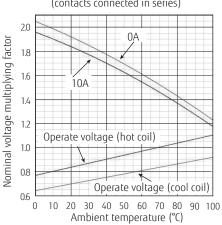
Note: When each contact is used independently, above graph shall be read; same voltage is applied on 2 coils, applied current 10A is 10A apply on each contact set.
