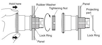
When the panel cutout dimension is 25 dia., remove the supplied rubber washer and mount the 25-dia. Ring as shown below. (Since the A22Z-R25 is not attached to the main body, order separately.) When using a Legend Plate (Order Separately), do not remove the rubber washer.
