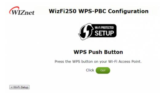
If you click the <Go> button on this web page, WizFi250 will scan the Access-Point in order to connect to it. The Access-Point must be set with <WPS-PBC> function as in this picture.
