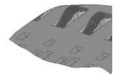
Contact design - the geometry of the contact has an important bearing on its electrical performance. Our contacts are designed to give an efficient wiping action and to maximize the stress between contact and card, so minimizing the contact resistance. The "spooned" contact area is also shaped so as to protect it from damage during card insertion.
