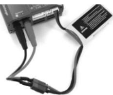
Failure to connect as shown in this diagram will damage this charger. To avoid short circuit between the charge lead always connect the charge cable to the charger first, then connect the battery. Reverse the sequence when disconnecting.
