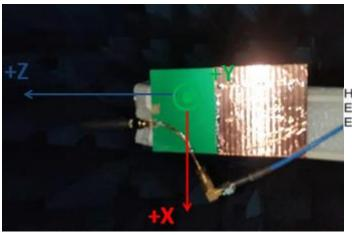
H plane: the tangent of XY E1 plane: the tangent of XZ E2 plane: the tangent of YZ
