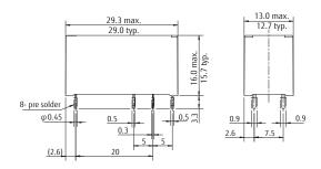
\*Dimensions of the terminals do not include thickness of pre-solder.
