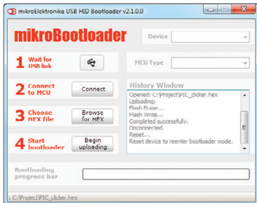
Figure 4-8: mikroBootloader ready for next job
