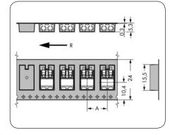
L = (pole no. x pin spacing) - 0.1 mm
