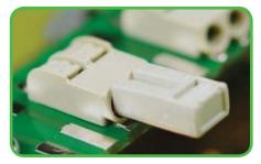
2000-402 Shorting Bar – used to complete the circuit at the end of a string of linear LED modules, e.g., insert with WAGO logo facing upward, and at a slight angle so the bottom of the housing clears the bottom edge of the terminal block wire entry opening.
