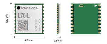
Quectel L76-L GNSS module supports concurrent reception of GPS, GLONASS (or BeiDou), Galileo and QZSS. It can acquire and track any mix of GPS, GLONASS (or BeiDou), Galileo and SBAS signals. The L76-L is designed to be compatible with Quectel L70, L76 and L76-LB modules, allowing convenient migration between them.
