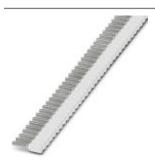
Taped ferrules, 0.5 mm², sleeve length 8 mm, with plastic collar, according to DIN 46228-4, white, for processing with the CRIMPFOX 4 IN 1, 10 strips each with 50 sleeves per strip.
