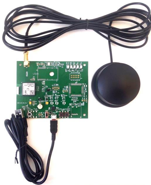
Figure 2: EVB and Accessories Assembly
