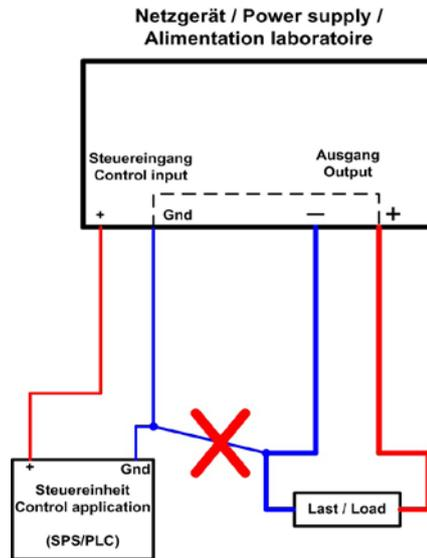
In order to measure the voltage at the load, use and wire the „Remote sense“ feature. The actual value output UMON, represents the voltage on the load and can be wired with the control application to measure the voltage. This prevents the current flowing via the control resp. measure lines.
