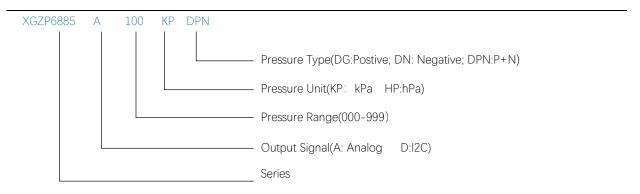
Note: 1. Voltage 5Vdc as default value, add 33(or 30) behind model signify 3.3V(or 3.0V) power supply, e.g.: XGZP6885A050KPDG33.
