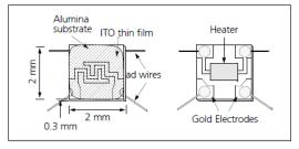
Fig 1. Sensing Elements
