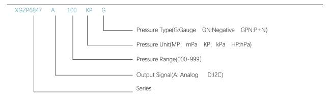
Note: 1. Voltage 5Vdc as default value, add 33(or 30) behind model signify 3.3V(or 3.0V) power supply, e.g.: XGZP6847A040KPG33.
