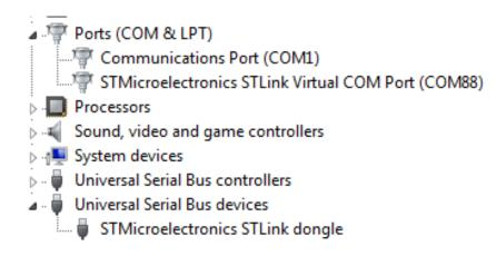
Figure 9: ST-LINK Interface Displayed on PC
