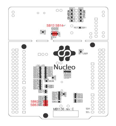
Figure 8: STM32-Nucleo Modification Diagram (Bottom View)
