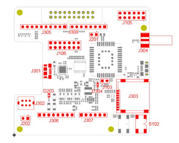
The following figure shows an interface distribution diagram of BC68-TE-B.
