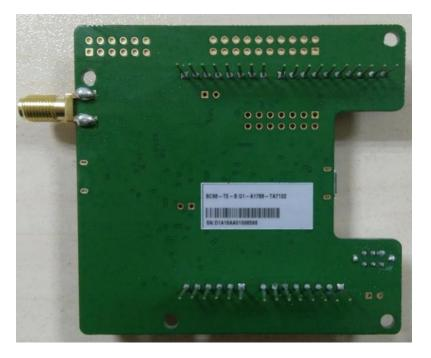
Figure 13: Bottom View of the BC68-TE-B
