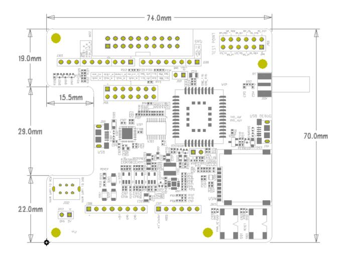
Figure 11: Dimensions of BC68-TE-B (Top View)
