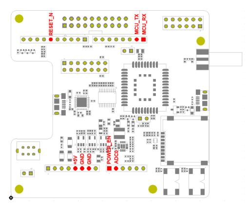
Figure 3: Pin Definition of Arduino Interface
