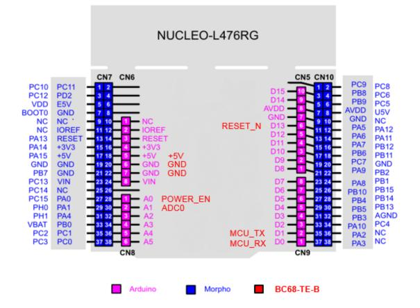
Figure 10: Pin Connection between BC68-TE-B and STM32-L476RG MCU
