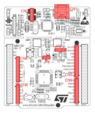
Figure 7: STM32-Nucleo Interface Diagram (Top View)
