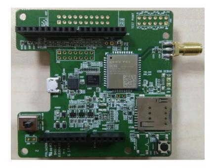
Figure 12: Top View of the BC68-TE-B
