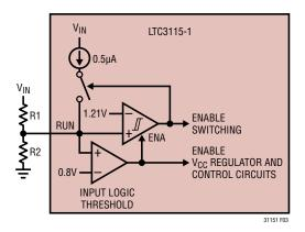
Figure 3. Accurate RUN Pin Comparator
