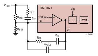
Figure 2. Error Amplifier and Compensation Network
