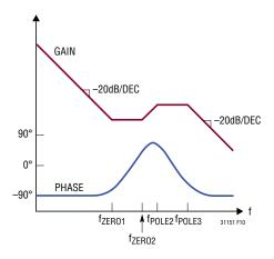
Figure 10. Type III Compensation Bode Plot
