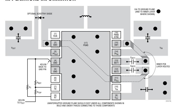
Figure 16. PCB Layout Recommended for the DHD Package
