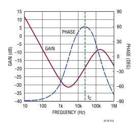
Figure 13. Compensated Error Amplifier Bode Plot
