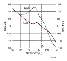
Figure 14. Complete Loop Bode Plot
