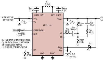
\*OPTIONAL-INSTALL D1 FOR IMPROVED EFFICIENCY AND LOWER INPUT OPERATING VOLTAGE
