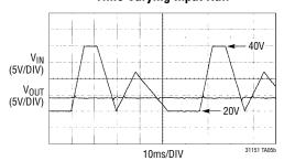
0A to 1.5A Load Step,  $V_{\text{IN}}$  = 20V
