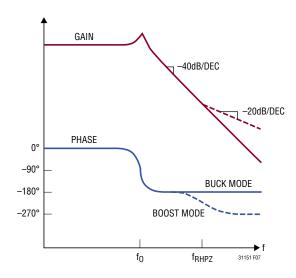
Figure 7. Buck-Boost Converter Bode Plot
