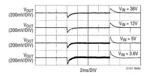
$V_{OUT}$  Transient for a OA to 2A Load Step,  $V_{IN} = 24V$
