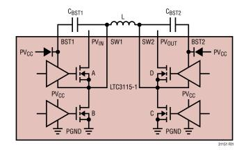
Figure 1. Power Stage Schematic
