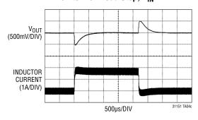
OA to 1.5A Load Step,  $V_{IN} = 10.6V$
