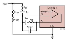
Figure 9. Error Amplifier with Type III Compensation
