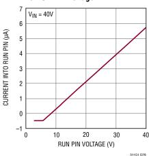
Shutdown Current on V<sub>IN</sub>/PV<sub>IN</sub> vs Input Voltage
