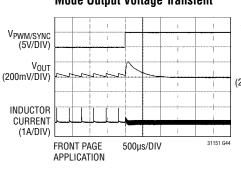
Phase-Locked Loop Acquisition, V<sub>IN</sub> = 24V 1.2MHz Clock
