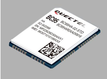
BC95 is a high-performance NB-IoT module with extremely low power consumption. The ultra-compact 19.9 × 23.6 × 2.2mm profile makes it a perfect choice for size sensitive applications. Designed to be compatible with Quectel GSM/GPRS M95 module in the compact and unified form factor, it provides a flexible and scalable platform for migrating from GSM/GPRS to NB-IoT networks.
