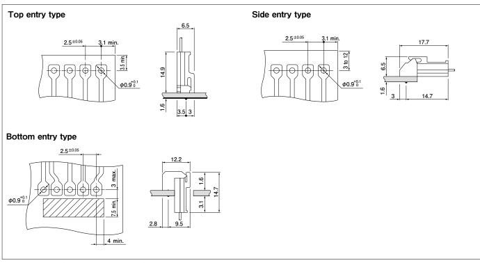
Note: 1. The above figure is the figure viewed from the connector soldering side. 2. Tolerances are non-cumulative:  $\pm$  0.05 mm for all centers.
