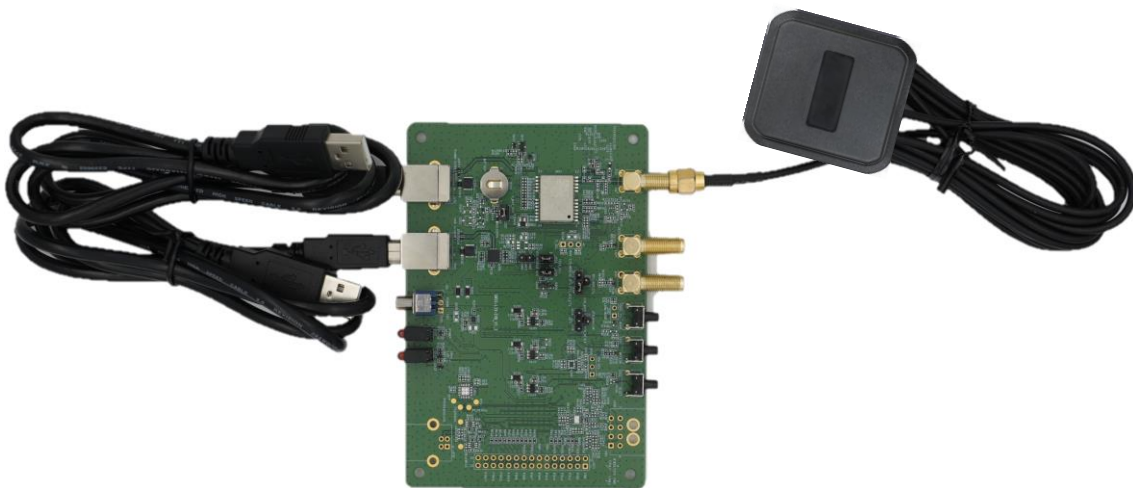
Figure 2: EVB and Components Assembly
