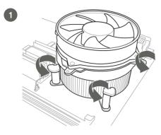
To uninstall the CPU heatsink and fan assembly
