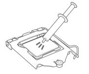
**CAUTION!** Apply the Thermal Interface Material to the CPU heatsink and CPU before you install the heatsink and fan if necessary.
