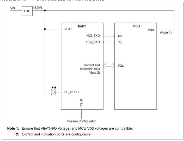
FIGURE 2-11: BM71 MODULE TO MCU INTERFACE
