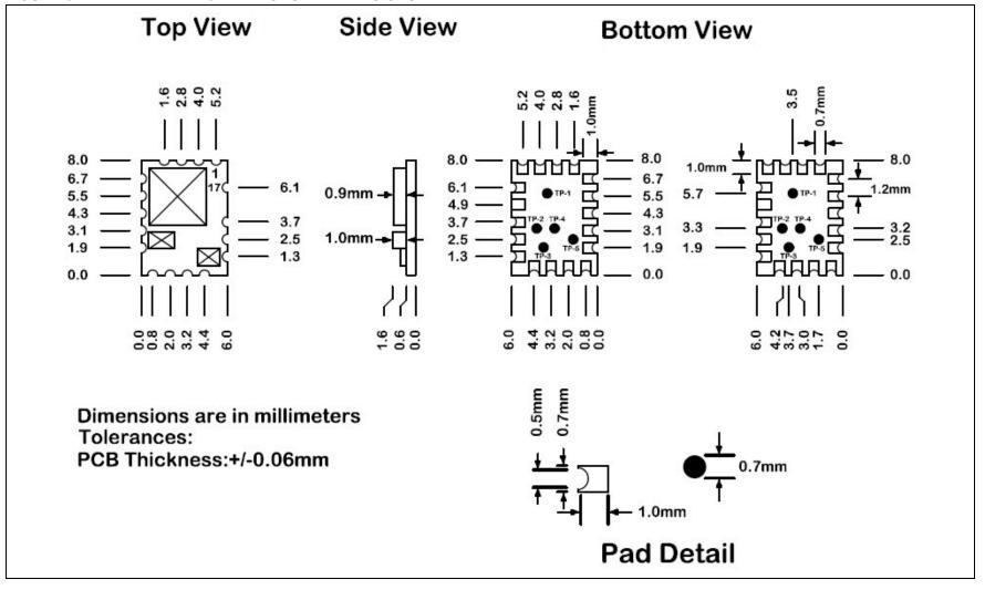
Figure 6-8 illustrates the recommended PCB footprint.
