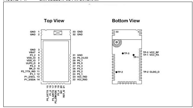
FIGURE 1-5: BM71BLE01FC2 PIN DIAGRAM
