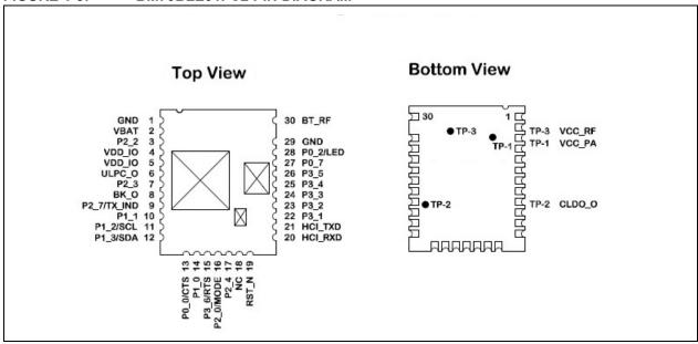
FIGURE 1-4: BM70BLES1FC2 PIN DIAGRAM
