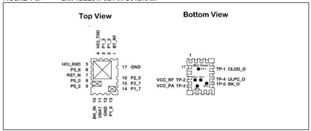
FIGURE 1-6: BM71BLES1FC2 PIN DIAGRAM
