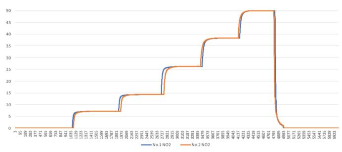
Test result: 50ppm full scale linearity error <± 5%;
