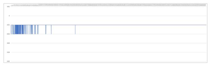
Test result: 12 hours clean air test, zero drift <0.02ppm (0-0.02ppm is the normal zero fluctuation range);
