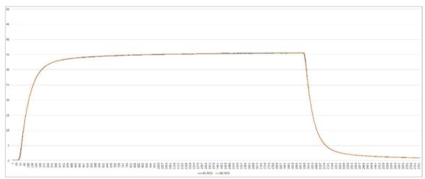
Test results: 2 hours ventilation, range drift <0.02ppm;
