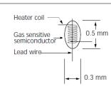
Fig 1a. Sensing element
