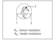
Fig 1d. Equivalent circuit
