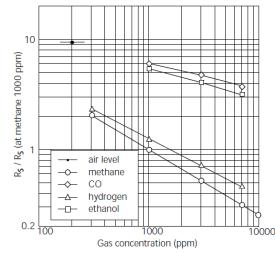
Fig3. Sensitivity characteristics
