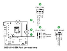
**CAUTION:** Do not forget to connect the fan cables to the fan connectors. Insufficient air flow inside the system may damage the motherboard components. These are not jumpers! Do not place jumper caps on the fan connectors!
