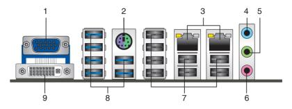
1. Video Graphics Adapter (VGA) port. This 15-pin port is for a VGA monitor or other VGA-compatible devices.
