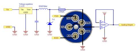
Fig. 1 Example schematic for Interfacing Integrated IR (INIR2-ME5%)
