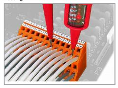
Testing via contact area above the conductors.
