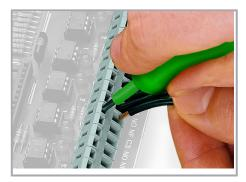
Inserting a conductor via 3.5 mm screwdriver.
