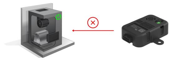
The sensor is equipped with a douple pole double throw (DPDT) electromechanical relay. The COM contact of one of the poles is connected to the sensor supply power pin. As a result, the relay pins can be under tension. Connecting without a suitable load may lead to excess current on the relay and permanently damage the relay.
