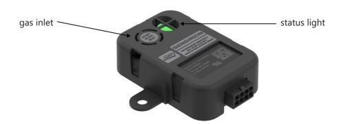
At the gas inlet, the sensing components are protected by a water, oil and dust protection membrane, situated below the "DO NOT BLOCK INLET" marking on the mounting bracket. Do not spray material on the gas inlet, as it may block the permeability of the membrane. A blocked membrane may inhibit the sensor from detecting a refrigerant leak. Do not mechanically or chemically damage the membrane, as it may result in failure of the sensing components.
