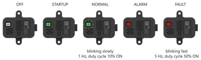
The status light indicator can be switched off completely through the Modbus interface, as described in the sensor datasheet.
