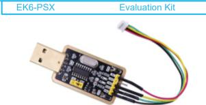
The main purpose of the Evaluation Kit is to install software that allows the user to read data from SGX Sensortech sensor module boards.
