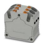
Distribution block, internally jumpered, connection method: Push-in connection, number of connections: 18, cross section:0.14 mm² - 1.5 mm², AWG: 26 - 16, width: 37.8 mm, height: 17.6 mm, color: black/yellow, mounting type: Direct mounting with flange
