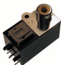
OTJ-6/ORJ-6 Dual SPDIF RCA and Optical Transmitter and Receiver Jack. Right angle PCB mount with self tapping hole for panel mounting. Hinged shutter. Several different colored inserts available.
