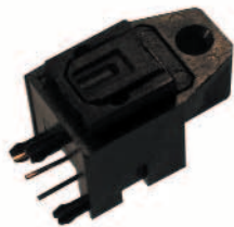
OTJ-5/ORJ-5 Single Optical Transmitter and Receiver Jack. Right angle PCB mount with self tapping hole for panel mounting. Hinged shutter.
