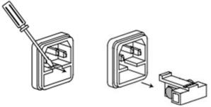
3. Replace the fuse with a new one, install it into the fuse box, and push the fuse box back on to the rear panel.
