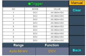
**3.** Clear the manual record: Press the Clear soft key to clear all data in the data table.(Note: because manual and automatic records share the same data table, automatic readings are also erased.).
