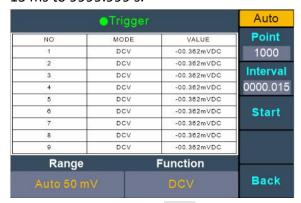
2. Record data: Press the Start softkey to start auto record. The loop icon will show up on the top of the display. Press the Stop softkey to stop recording, the data table shows the readings taken. press keys to turn the page.
