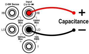
**Tip:** Please short contact the two feet of an electrolytic capacitor by using a test lead before measuring the electrolytic capacitor.
