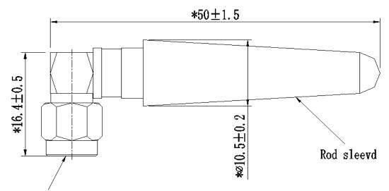
SMA/Au-PLATED (Male pin with internal thread) Salt spray requirements: ≥48h
