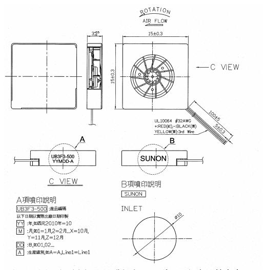
Sunon standard sample exclude the connector. If there is any request for connector, please advise in advance. About recommend connector, SUNON recommend the following models for SUNON Mighty Mini Fon/Blower: 1.(JST) SUR series connector: 02SUR-32S / 03SUR-32S.
