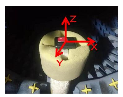
H plane: the tangent of XY E1 plane: the tangent of XZ E2 plane: the tangent of YZ
