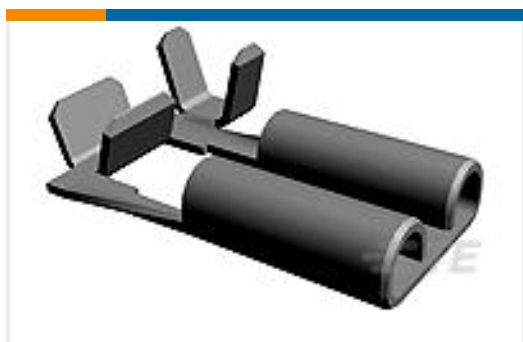
TE Part #1742086-2 187 FASTON, FLAG, REC., 18-22 AWG, TPBR
